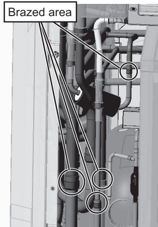
Removal of the front heat exchanger on a high-efficiency model (Figure 8)
