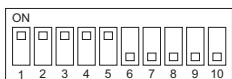
The figure at left shows that the switches 1 through 5 are set to ON and 6 through 10 are set to OFF.
