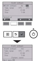
Move the cursor to the desired item with the F1 or F2 button out of Night setback No (disable)/Yes (enable), Temp. range, Start time, or Stop time.
