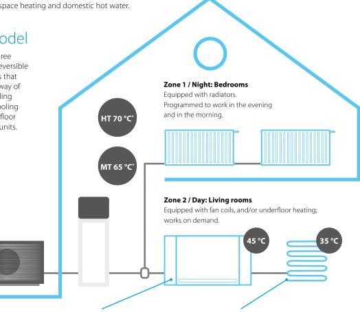
**Daikin Altherma HPC** (heat pump convectors) are hydronic emitters that can provide cooling or heating. They can be combined and are a perfect fit with underfloor systems.
