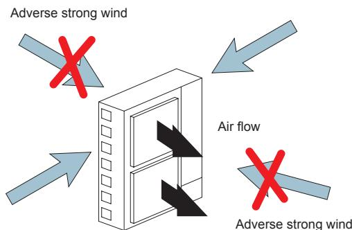
Strong winds against the unit's air outlet causes short circuits and these can be the consequences:
