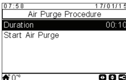
After "Test Run" or "Air Purge" option is selected, the YUTAKI user controller asks for the duration of the test.
