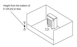
C) Create an appropriate ventilation open area. Make sure that the width of the open area is 0.9 [m] or more and the height of the open area is 0.15 [m] or more. However, the height from the bottom of the installation space to the bottom edge of the open area should be 0.125 [m] or less. Open area should be 75% or more opening.
