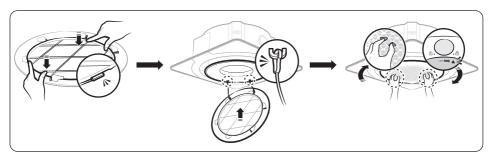
After cleaning and reassembling the air filter, reset the filter-cleaning reminder as follows:
