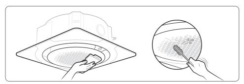
Wipe the surface of the unit with a slightly wet or dry cloth when needed. Wipe off dirt from odd-shaped areas by using a soft brush.
