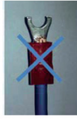
Terminal has been cut.
